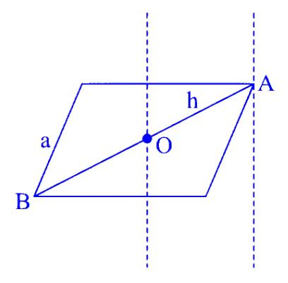
$$\begin{split} I_{O} &= \frac{Ma^{2}}{6} \\ AB &= \sqrt{2a^{2}} = \sqrt{2}a \\ \therefore \quad AO &= \frac{a}{\sqrt{2}} = h \\ \therefore \quad I_{A} &= I_{0} + Mh^{2} \\ &= \frac{Ma^{2}}{6} + \frac{Ma^{2}}{2} \\ &= \frac{8Ma^{2}}{12} = \frac{2}{3}Ma^{2} \end{split}$$
